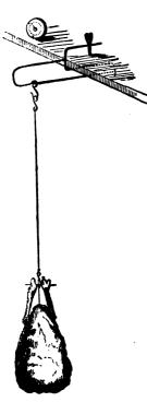
This represents a model of a Chimney Screw-jack for suspending joints to. Its cost is very trifling, and may be purchased at any ironmonger's. It will fit on any mantel-shelf; and it enables the joint to be shifted nearer or further from the fire, as occasion requires.
