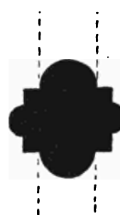
Fig. 333.—Stradella. Church of Montalino. Section of pier (Xth Century).
