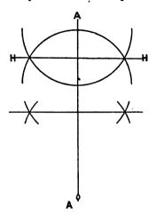
passes half round on the under side: then put the leg of the compasses on the point of intersection of these two lines 2 and make the other halfcircle above, and you will always find a cross on your right hand by the lines intersecting each other. Do same on the left hand. which will give you two
