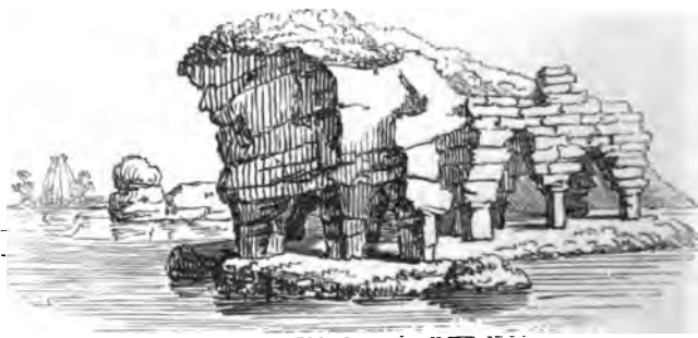
[Fig. 134. Imaginary sketch, exhibiting the principle of perpendicular pressure in the artificial vaults made in the native rock in India, and also in the arches of buildings in the Indian style, and even in their domes. See the elongated dome in the background of the vignette.]
