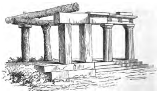
[Fig. 132. Sketch exhibiting the progress of Grecian architecture, from the columns and beams formed of the trunks of trees, with the bark on, to the Doric order, with fluted shafts, &c.]
